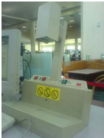
Bar code reader and strip magnetiser combined
